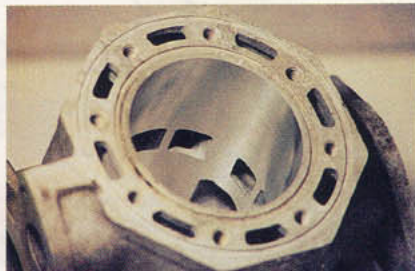
The cylinder is then bored to return it to exact specifications before replating.
