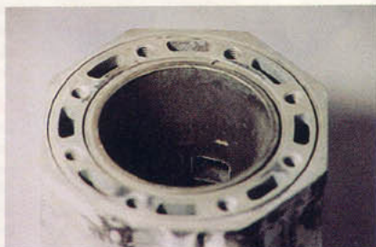
Once the cylinder is replated, the process is not complete; note the extra material in the port areas.
