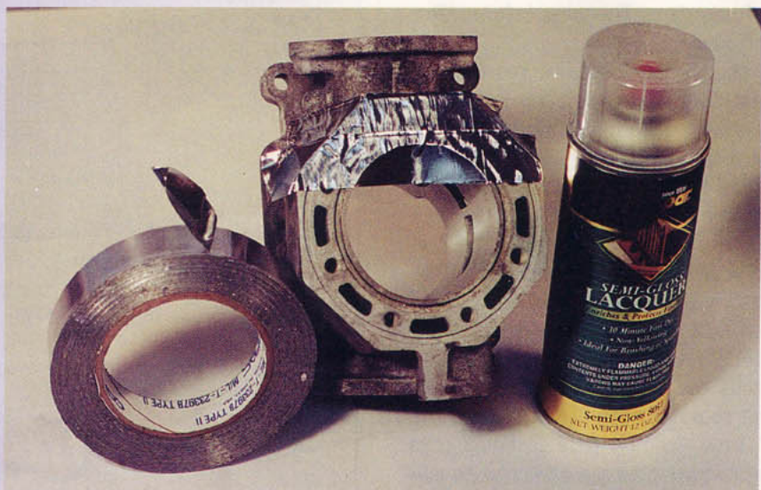
Lacquer is used to protect the cylinder during the process of removing the damaged plating with acids & caustics. Aluminum tape is then used to mask the head surface during the replating process to protect the areas that are not to be coated.
