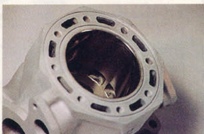
After precision honing, the finished product is ready to return to service.
