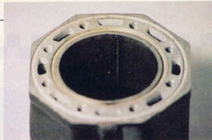
This plated cylinder has damage which requires the plating to be removed.
